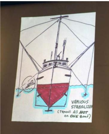
**Tom Stevens** gave a detailed dissertation on the shape of hulls as related to stability concerns. Such factors as the curve of the hull, its depth, rolling chocks, boom stabilizers, and gyro - controlled fins are
