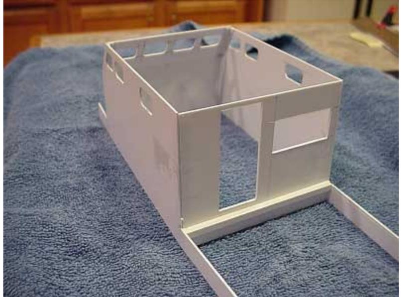
If you notice the picture on the right, I used angle pieces at each corner and I ran the angle piece the entire length. This not only provided me a guide to keep the edges aligned but also provided a very strong support bracket to glue to. In addition to this you'll also notice that I glued on a floor piece. This also has angle support brackets on the bottom. This gave me the lateral strength that I needed to prevent the pilothouse from moving sideways.
