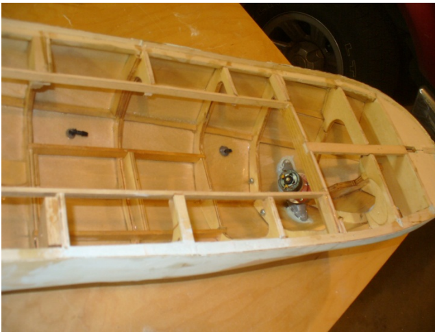
Bow thruster and water inlets installed in hull
