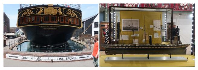
When the SS Great Britain was built she was the longest passenger ship in the world from 1845 to 1854. The ship measured 98 meters long, almost 10 meters high and had a propeller almost 5 meters (16 feet) in diameter.
