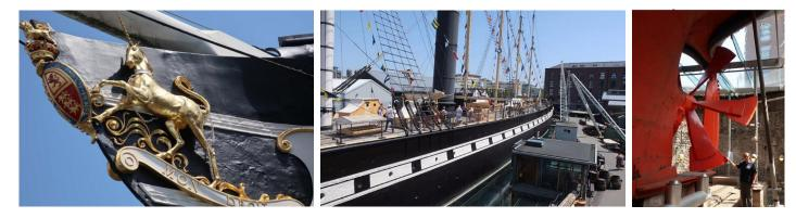
She was designed by Isambard Kingdom Brunel; Mr. Brunel was a great inventor. He was the first to use a balanced rudder, which is a rudder with the rudder post part way back on the rudder which makes it easier to turn, he designed this ship.
