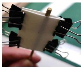
Use some styrene solvent dripped down the inside of the front and rear edges of the rudder. Do this a little at a time so you do not soften the sides of the rudder or dissolve the back inner sides of the rudder more than to just weld the two pieces together.
