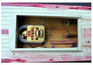
holding it in place. I decided to fix the other connections by cleaning the wire right next to the battery holder and then solder the wire to the holder since the holder is made of brass. It is now working. I need to reattach the hardware and it is ready to run.
