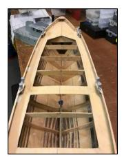
After I completed the hull the deck was added. Note that some frames were made from  $\frac{1}{4}$ " plywood to make things a little more stout.
