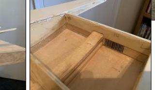
I started building the hull, but reading about the CQ, found she rode really low in the water. I chose to add a half inch of depth to the hull. It caused no ends of difficulties, bolt with the frame and with the skin. I finally got it, and with the exception of the bow stem, it came out all right.
