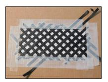
The trick was how to make the weave in the middle and attaching it. First solution was to make the netting weave that goes in the middle out of masking tape. This would require taking a length of tape, folding sticky
