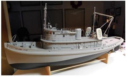
Here is my current project, the US Army tug LT157, a Miki Miki Class tug that was built at Northwestern Shipyard in Bellingham back in WW2. This started as a Gary King semi kit that I won at the 2014 regatta. It is a fiberglass hull and deck with the basic house made from laser cut plywood. The rest of the boat has been modified with a lot of scratch built parts.
