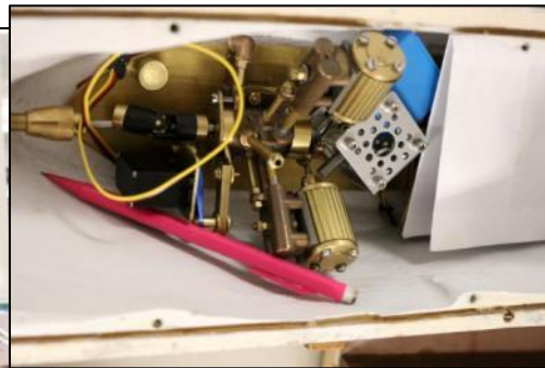
He was advised not to build the superstructure out of styrene due to heat buildup from his steam plant. He will most likely build it out of plywood now. He also showed some very small cameras which he plans to install next to the pressure and water level gauges next to his steam plant since they cannot be viewed openly.
