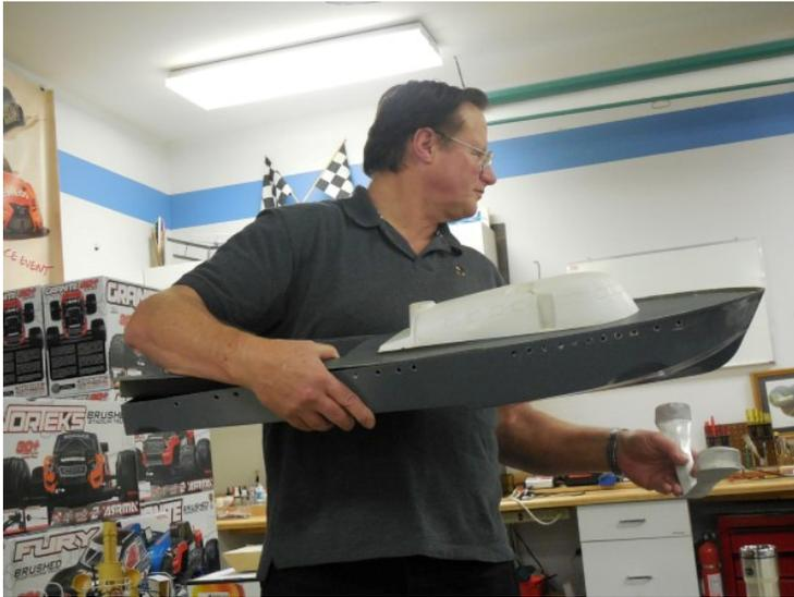
**Phil Northrup** showed his miniature tug attached to a barge both of which have drive mechanisms. There are red lights which illuminate in reverse and white ones for forward motion. He has used fuel tubing for the universal joints.
