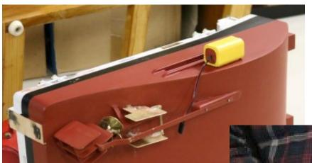
Bob Wickham demonstrated how he constructed the forward rudders to act in unison with the rear rudders, the posts of which penetrate the hull to be connected to the rudder horn and servo. There was not enough room in the hull to put in forward penetrating rudder posts. The dual prop super springer is really looking cool.
